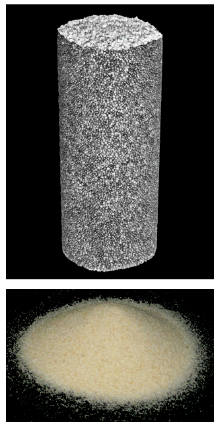
Fig. 5. Consolidated kRT 100 proppant pack (top), versus uncoated 100 mesh sand (bottom).
